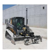
they could do. All that changed, however, with the addition of a 3D LPS (local positioning system) solution, which uses a fast-tracking Topcon GT Series robotic total station to register and maintain screed position from a machine-mounted prism and sonic tracker. Height adjustments — transmitted to and from the screed at a rate of 10 times per second — maintain even the tightest accuracies.
